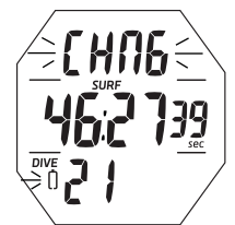
Fig. 73 - FREE SURFACE LOW BATT ALARM
