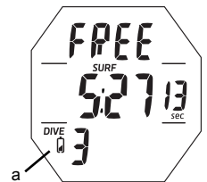
Fig. 2 - LOW BATTERY WARNING
